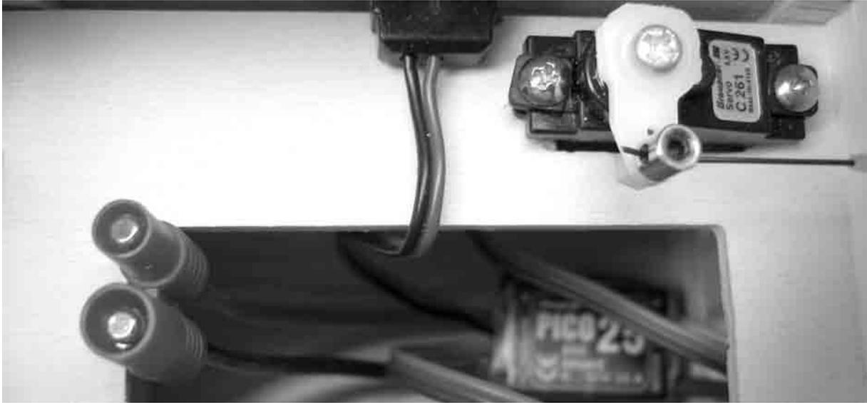
Install the PICO 25 speed controller below the battery compartment. The On / Off switch should be mounted in the left-hand fuselage side, as shown in the picture. Cut an opening in the fuselage side, and fix the switch in place using a drop of cyano.
