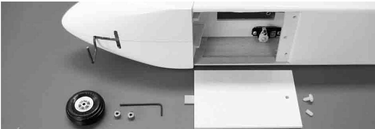
Fit the nosewheel on the axle and secure it using the collets supplied. The battery well cover is held in place with an M4 screw, shortened as shown.
