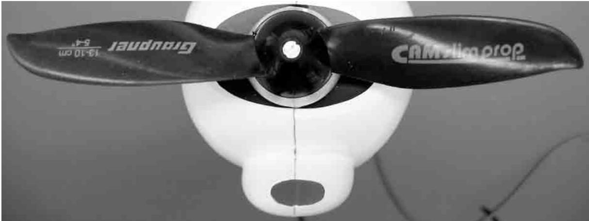
Cut out the front face of the air intake at the bottom of the nacelles, and apply the oval black decal to the front faces before installing the motors permanently. **Caution:** it is important to test-run the motors before gluing the nacelles to the wing: the static current drain should be around 4.1 A at 7.4 V, i.e. with two LiPo cells. **Caution:** if you subsequently switch to three LiPo cells, you must use smaller propellers, e.g. Order No. 1361.12.10.
