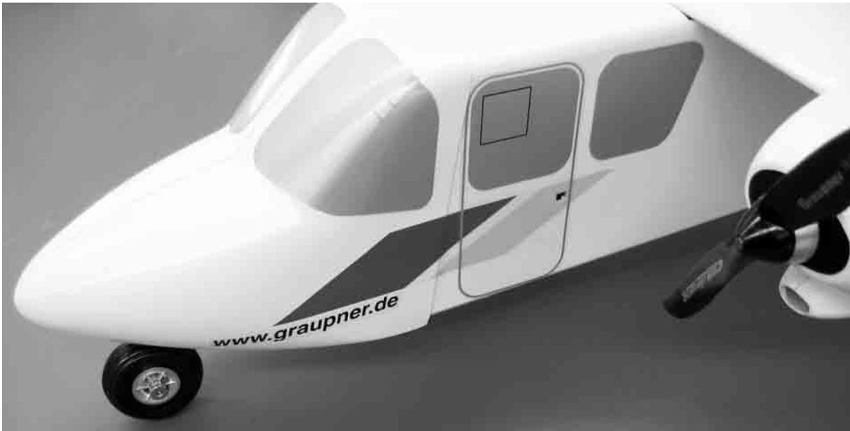
The final stage in assembling the model is to cut out and apply the decals. Please note that the front windscreen should be applied in two separate parts in order to avoid excessive wrinkles. Mark the dummy ribs on the strut fairings using a felt-tip pen.
