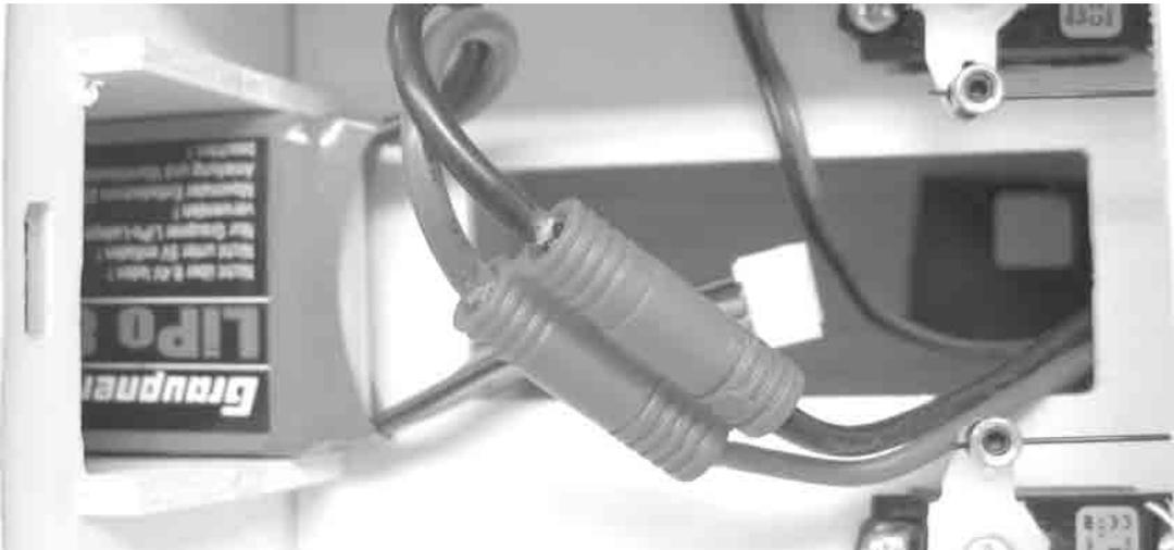
The LiPo battery fits in the battery compartment. Caution: make sure the speed controller is switched off before you connect the G3.5 connectors.
